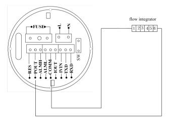
Figure 4.4.2 (c) Connection of Electronic Counter
