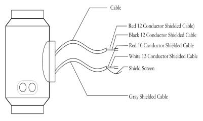
Fig.4.4.1Labels and connection of signal lines in circinal model Signal lines labels in circinal model:
