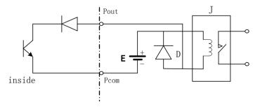
Fig.4.5 (c) Digital output connect relay
