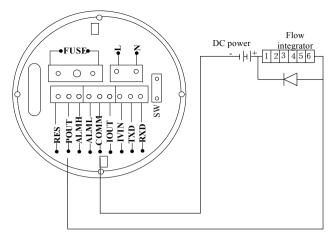
Fig 4.4.2(b) Connection of Electro-Mag 511Bnet Counter
