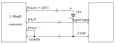
Fig.4.6 (b) L\_Mag 511 three connection( power supply and current output are not insulated)
