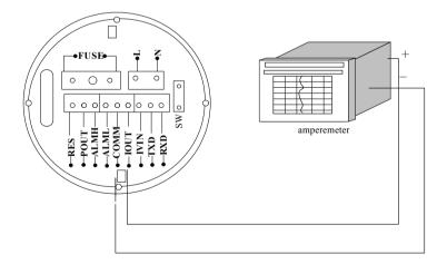
Fig.4.4.2(a) Output and power supply cables
