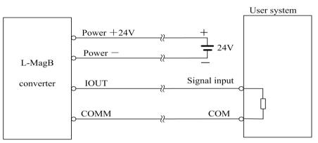
Fig.4.6 (c) L\_Mag 511 four connection( power supply and current output are insulated)
