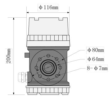
Fig.1.3 L-mag 511B series511C Shell
