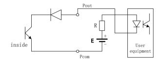
Fig.4.5(b) Digital output connect photoelectricity coupling
