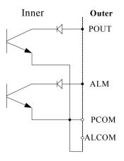
Fig.4.4.2(e) Connection of OC Gate
