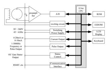
Fig.2. 1 Structure Of Converter's Circuit
